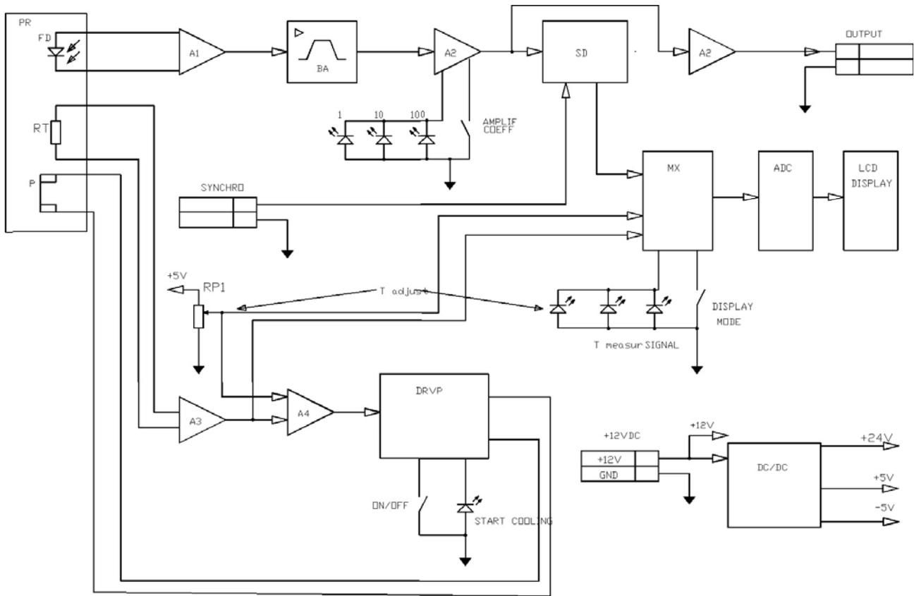
Fig. 12. The Block diagram of AMT-07.
