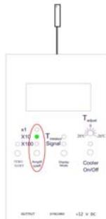
**Fig.10.** The button and indicators of discrete changing of current amplification.
