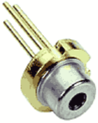
5.6 mm laser diode package
